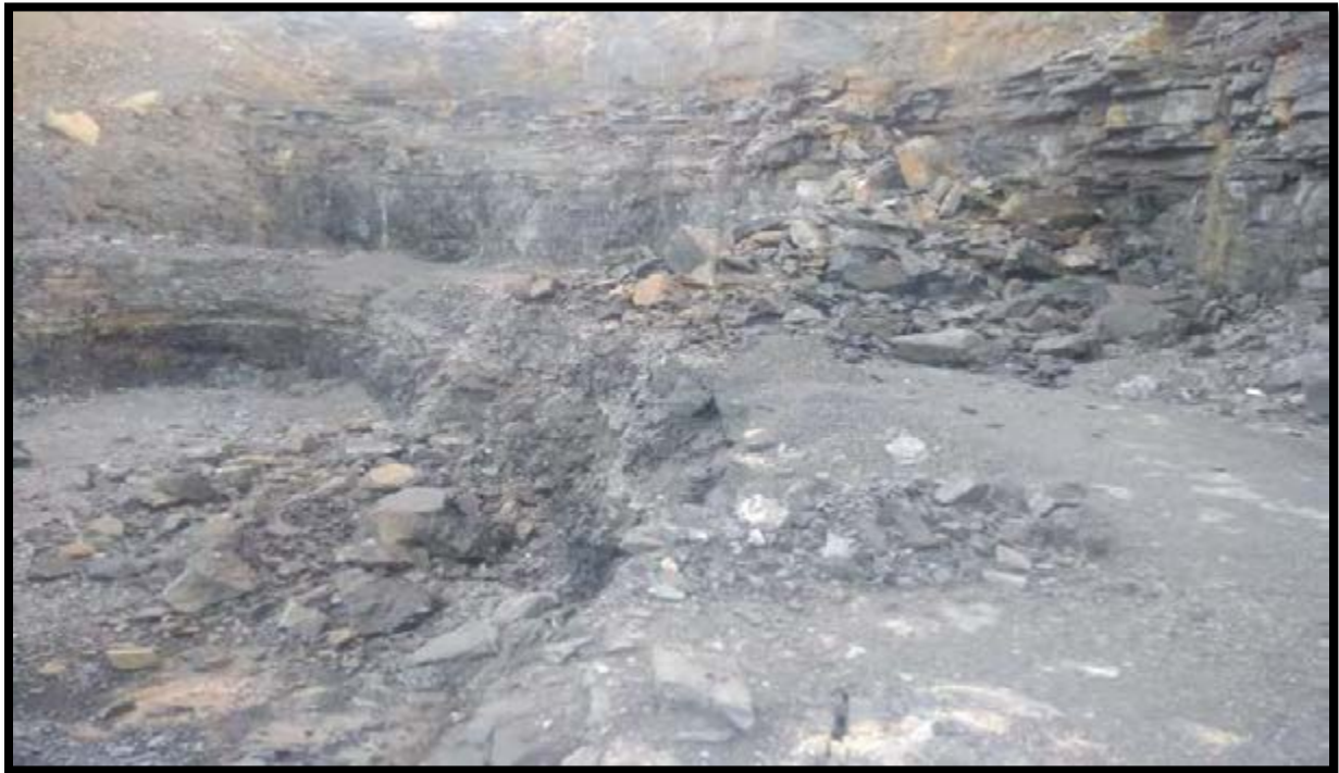
Fig.12: Flatter Muck pile Shape after Blasting
