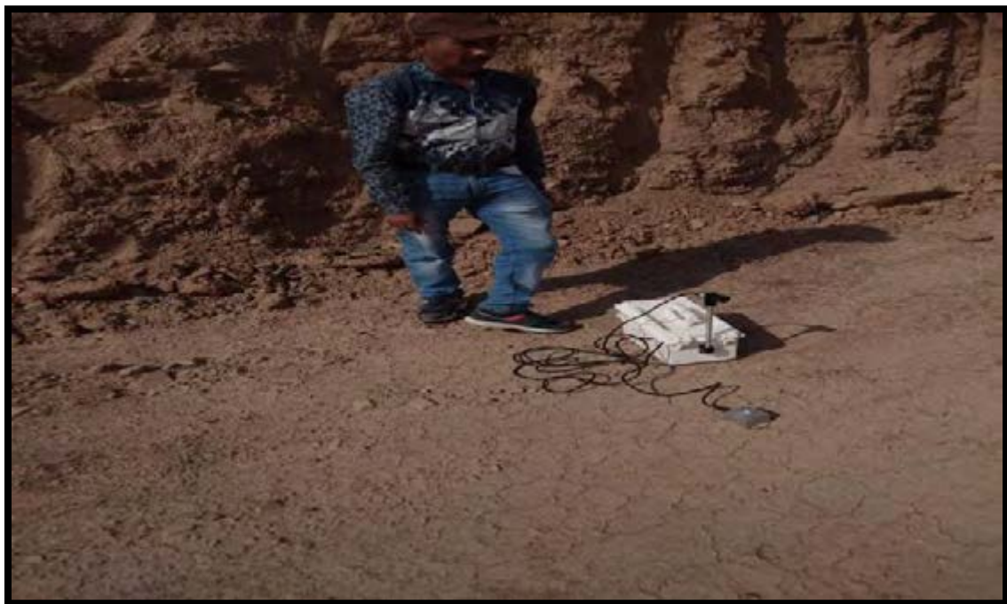
Fig.6 : Ground Vibration Monitoring Site at 10m Distance (Behind the Blast Site)
