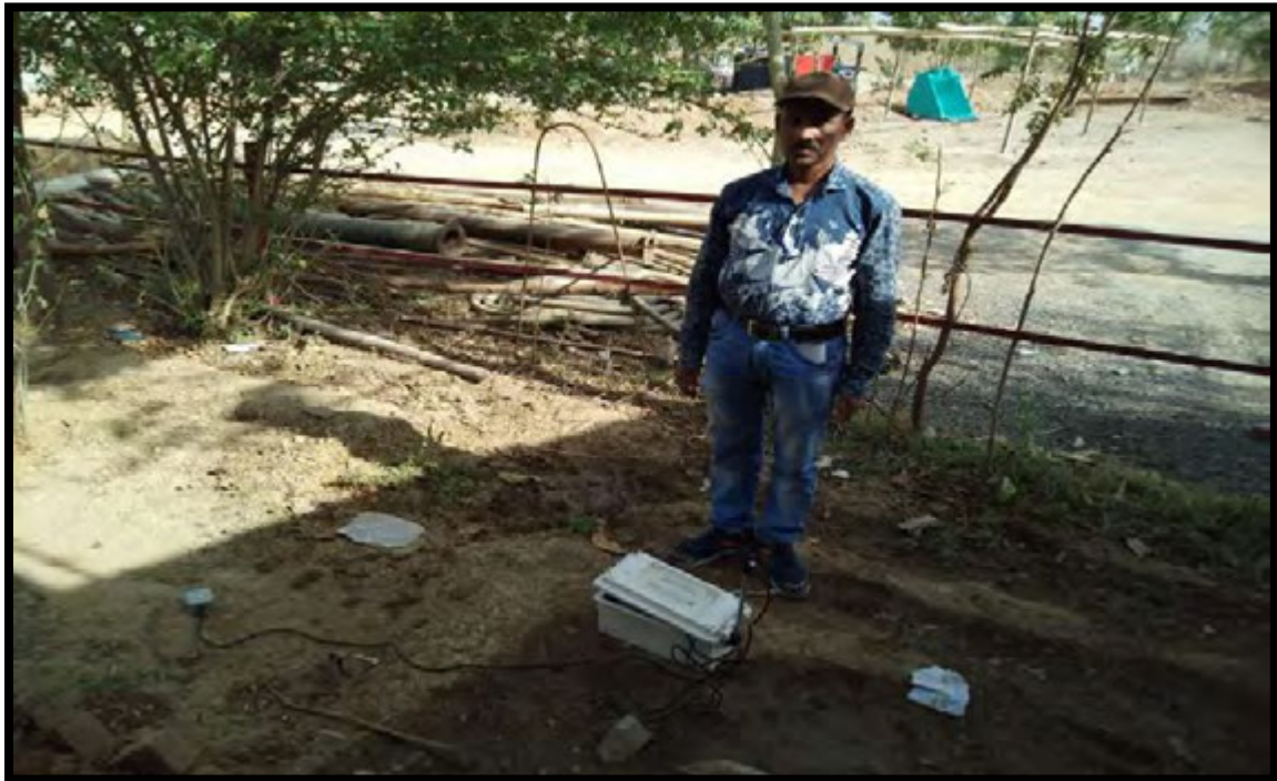
Fig.5 : Ground Vibration Monitoring Site at 350m Distance from the Blasting Site
