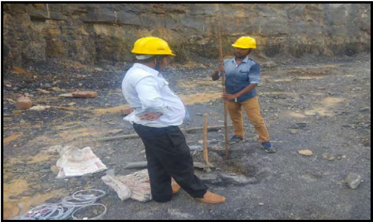
Fig.10: Stemming with Crushed Aggregate Material
