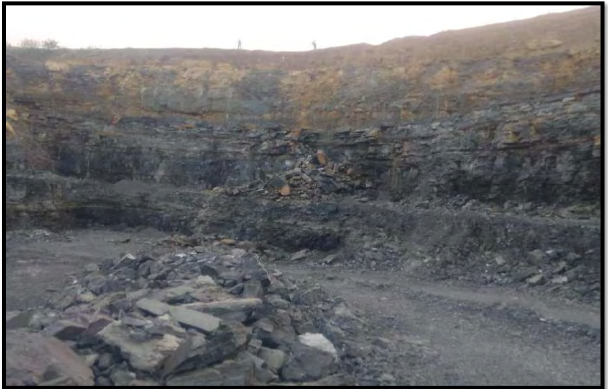
Fig.3: Bedding of Limestone and Dolomite Rock Stratum
