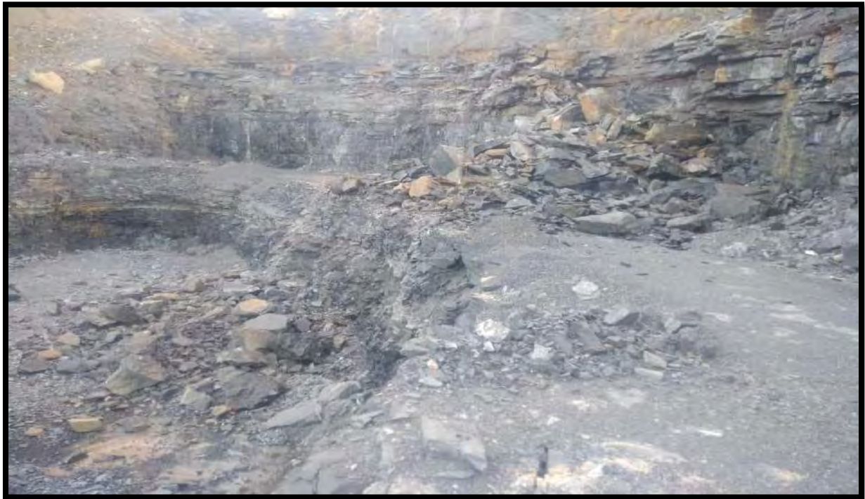
Fig.12: Flatter Muck pile Shape after Blasting
